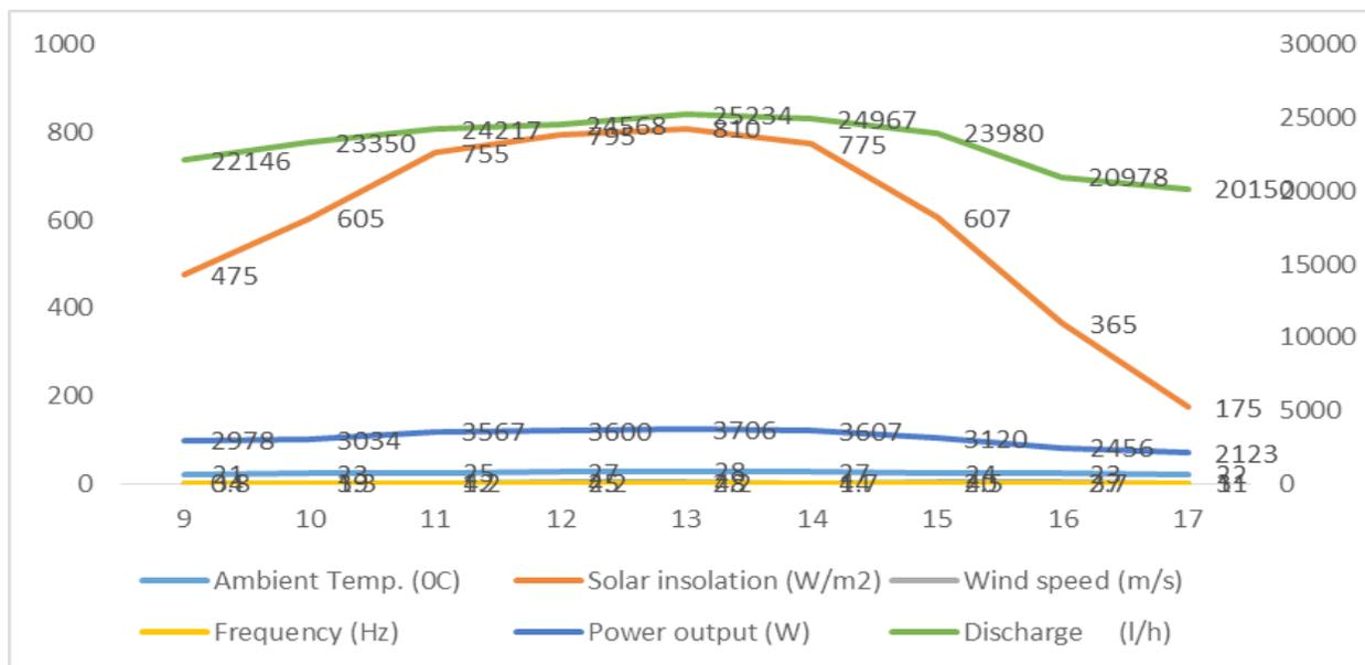
**Fig. 2: Performance of solar photovoltaic water pumping system with respect to weather parameters at farm-1.**
