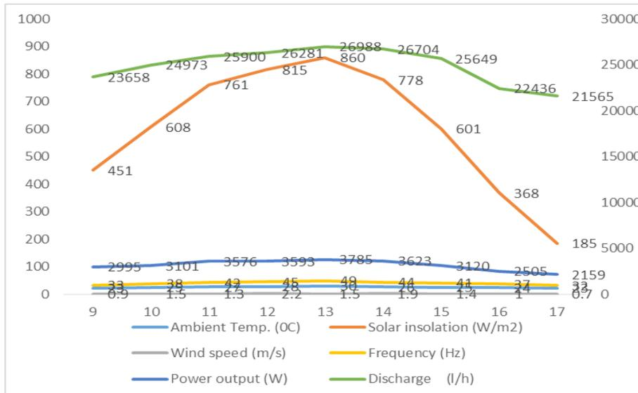
**Fig. 4: Performance of solar photovoltaic water pumping system with respect to weather parameter at farm -3**
