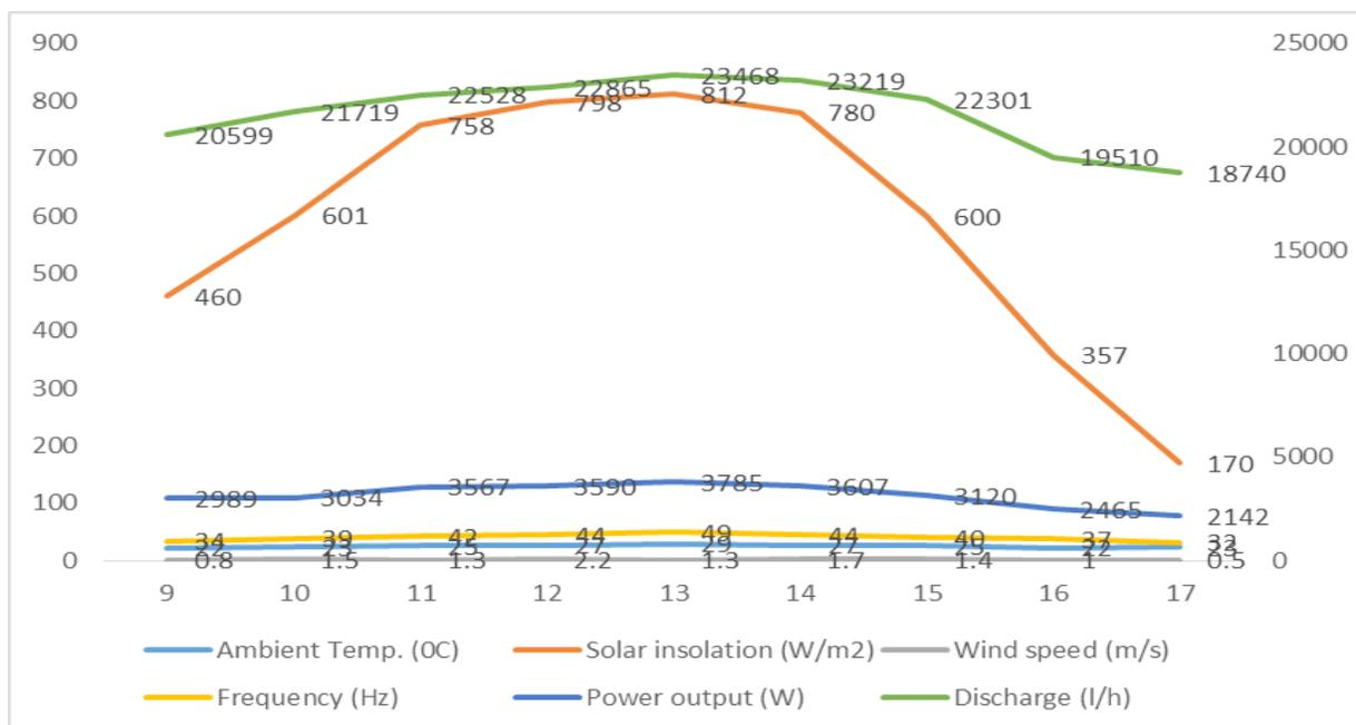
**Fig. 3 : Performance of solar photovoltaic water pumping system with respect to weather parameters at farm-2.**
