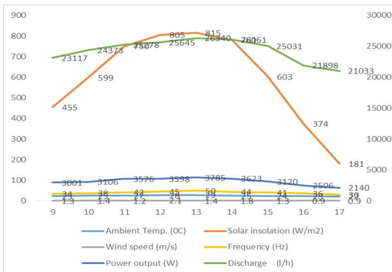
**Fig. 5 : Performance of solar photovoltaic water pumping system with respect to weather parameters at farm-4.**
