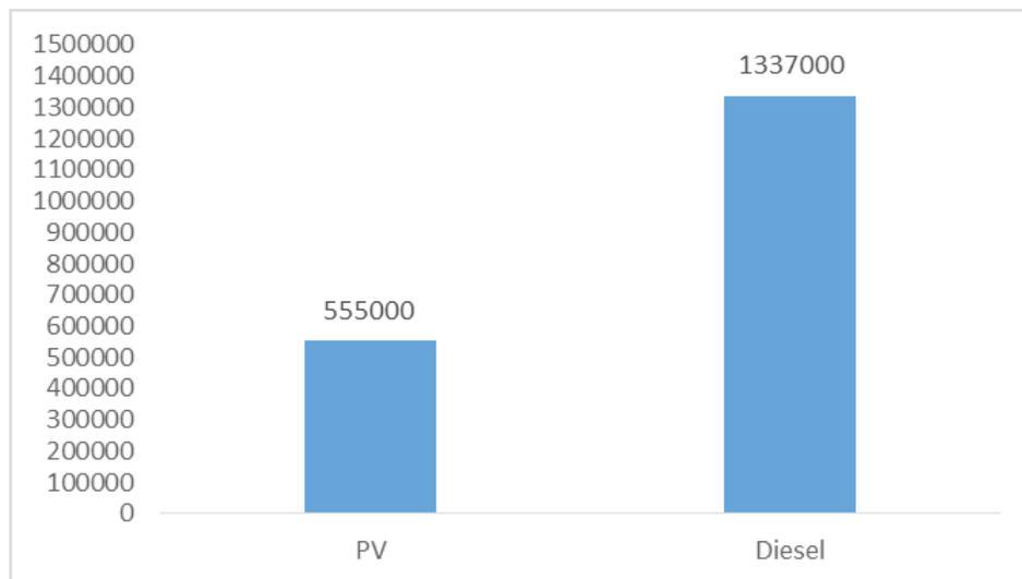
**Fig. 6: System cost comparison by life cycle cost analysis**
